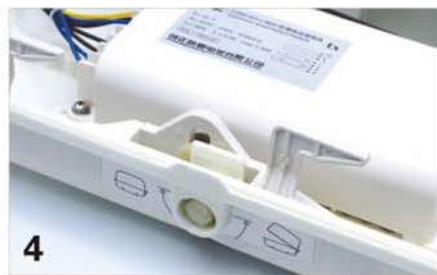
The enclosure and transparent shield are pressed tightly and drive the switching off and interlocking function of explosion-proof distance switch by unlocking device through interlock mechanism.
