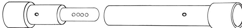
400 Amp 1.25" Solder Wire Well Terminals. Solid Copper Contacts with Four Spring-Loaded Borosilicate Bearings.
